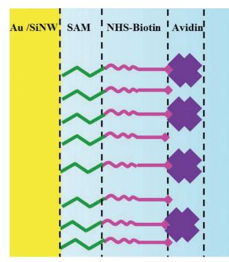
Figure 1. Schematic of the composite structure for avidin detection.
