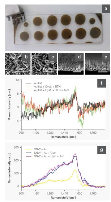
Figure 2. (a) Picture of the Au/SiNWs on a Corning<sup>®</sup> glass slide. SEM images of the SiNWs before (b and d) and after Au coverage (c, e). The images b and c are top view and d and e are side view. (f) Raman spectra of the modified Au film without SiNWs. (g) Raman spectra of the modified Au film with SiNWs.
