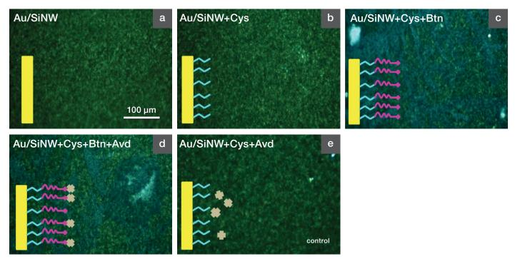
Figure 3. Optical images depicting each functionalization step obtained using a DXR3 Raman Microscope. A sketch illustrating each step is included in the corresponding image. (a) Pristine Au/SiNWs; (b) modified with cysteamine; (c) NHS-biotin functionalization; (d) immersed in avidin solution; and (e) a control experiment where the Au/SiNWs coated by sole SAM was immersed in the avidin solution.
