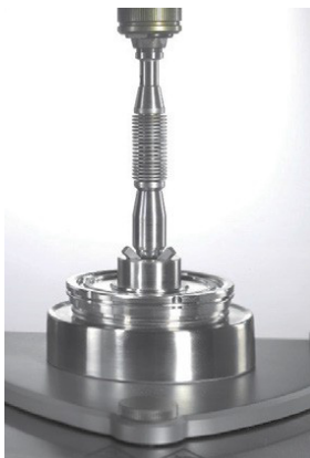
Figure 2: Tribology setup for HAAKE MARS iQ Rheometer based on the ball-on-3-plates principle.
