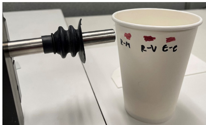
Figure 5. An in situ measurement of lipstick on a cup through the fiber probe accessory.
