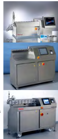
Overview of parallel twin screw extruders (top: Pharma11 with 11 mm, middle: Pharma 16 with 16 mm, and bottom: Pharma 24 with 24 mm screw diameter)
