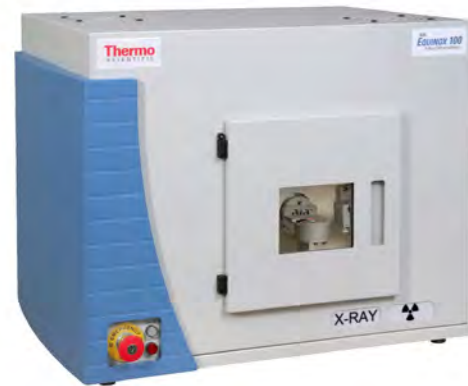
Powder sample holder in transmission configuration
