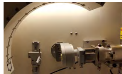
Powder sample holder in transmission configuration
