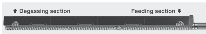
Figure 1: Set up of screws and barrel used for the scale-up experiments on the Pharma 11, Pharma 16, and Pharma 24. At the feeding section, the Soluplus is added, and the pigment is added at a given time T_0 . The degassing section at the left-hand side is an atmospheric degassing to allow water vapor to evaporate out of the polymer.
