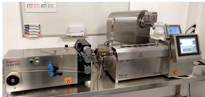
Figure 1: Benchtop system including a Pharma 11 Twin-Screw Extruder for production of ODFs.
