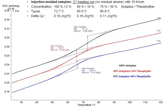
Figure 14: EDSC measurements — second heating run (10 K/min) with 3 injection molded samples with different Theophylline concentrations (0% black, 10% red, 30% blue) in Soluplus®.
