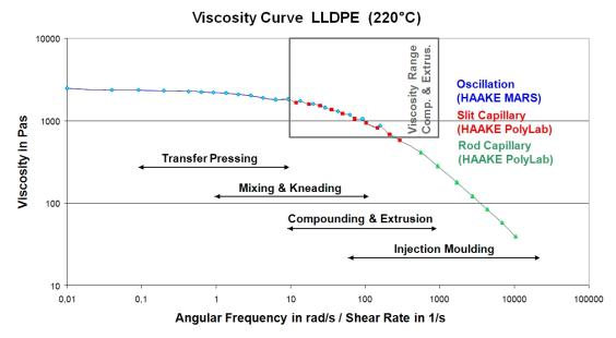
Figure 1: Viscosity curve of LLDPE and typical shear rate ranges in rheometry as well as in polymer processing.
