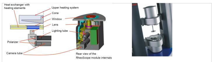
Figure 7: HAAKE RheoScope module: Schematic drawing (left: side view, center: rear view) and mounted in the HAAKE MARS rheometer (right).
