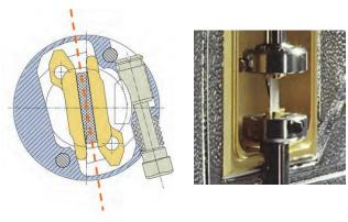
Figure 4: Self-centering and self-tightening spring-loaded DMTA solid sample clamps (drawing left) in a CTC oven and with an injection molded bar sample (right).
