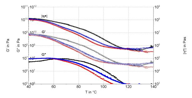
Figure 12: D heating run (5 K/min) with 3 injection molded rectangular bars with different Theophylline concentrations (0% black, 10% red, 30% blue) in Soluplus® measured with DMTA clamps (measuring amplitude: 0.01 %, measuring mode: CD-AS¹4).
