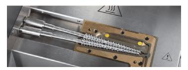
Figure 5: HAAKE MiniLab can be used with counter-rotating or corotating conical twin screws (center), has a bypass valve (right), a back flow channel with a slit capillary with two pressure sensors for viscosity measurement (top) and an extrusion channel (bottom right).
