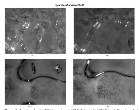
Figure 10: Powder mix with 20% Ibuprofen and 80% Soluplus® at 27 °C (top left) and gradual melting of the API shown in images taken at 75 °C, 85 °C and 91 °C (lens 20 x).
