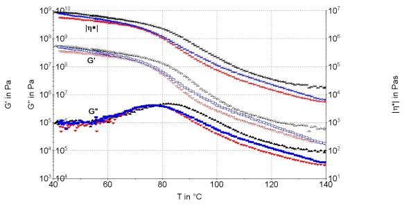
Figure 11: A cooling run (-5 K/min) with 3 powder samples molten at 140 °C with different Theophylline concentrations (0% black, 10% red, 30% blue) in Soluplus® measured in plate/plate measuring geometry (measuring amplitude: 0.01 %, measuring mode: CD-AS¹4).
