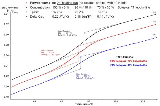
Figure 13: DSC measurements — second heating run (10 K/min) with 3 powder samples with different Theophylline concentrations (0% black, 10% red, 30% blue) in Soluplus<sup>®</sup>.
