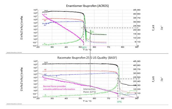
Figure 9: Heating runs (1 K/min) with Ibuprofen powder (top: enantiomer, bottom: racemate), chirality indicated symbolically top left (measuring amplitude: 0.1% with powder, first 10% then 30% with fluid, measuring mode: CD-AS<sup>14</sup>).
