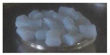
Figure 3: Extrudate pieces placed on the lower plate of the measuring geometry for melting and subsequent loading and trimming.
