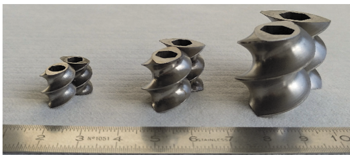
Figure 3: The three scales in this study: 11 mm, 16 mm, and 24 mm sized twin screws.
