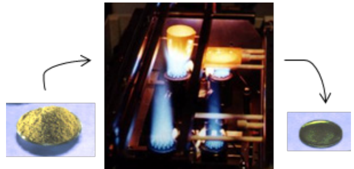
Figure 2: Transformation of the powder material into a glassy sample by fusion at high temperature.
