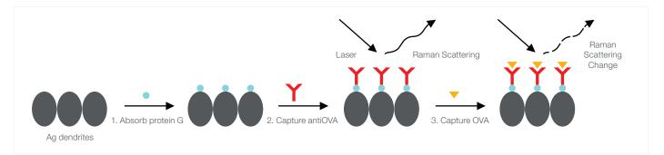
Figure 2. The preparation of the modified silver dendrites and SERS analysis of the bound protein.
