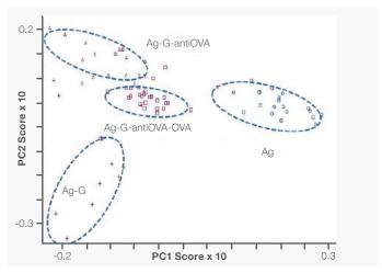
Figure 4. PCA plot of spectra from the different steps of the modified silver dendrite process.
