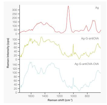
Figure 3A. Average spectra of the bare silver dendrite, silver dendrite with bound protein G and antiOVA (Ag-G-antiOVA), and silver dendrite with protein G, antiOVA, and captured OVA (Ag-G-antiOVA-OVA).
