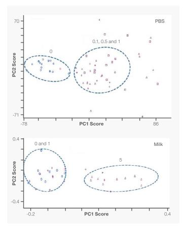
Figure 5. PCA limit of detection (LOD) plots for OVA in PBS (top) and OVA in milk (bottom).
