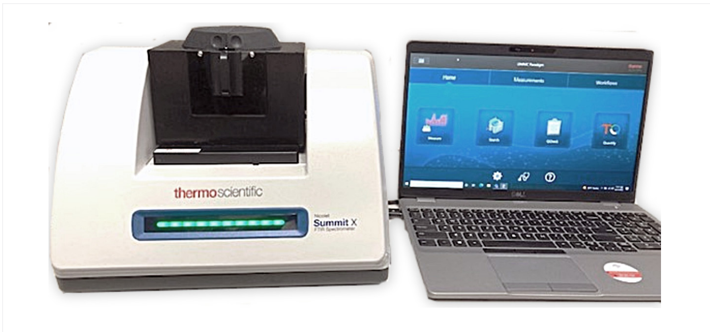
Figure 1. Nicolet Summit X spectrometer with Collector II accessory.
