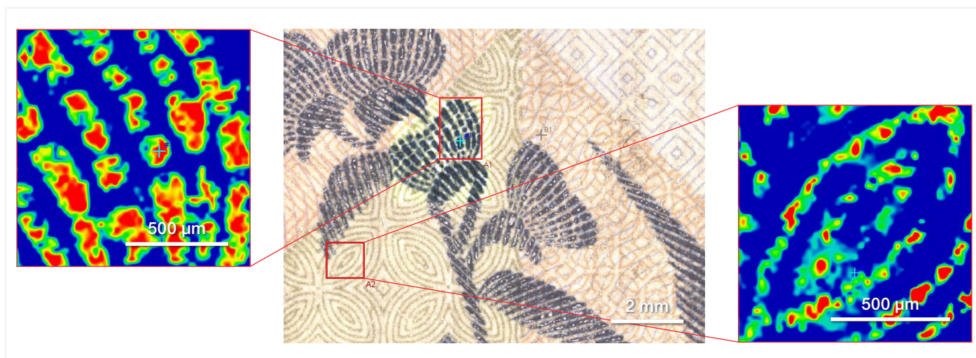
Figure 3. Infrared images generated from the printed designs on a banknote. Peak area images were generated for the flower, using a calcium carbonate peak at 871\text{ cm}^{-1} (left), and the background pattern, using a carbonyl peak at 1735\text{ cm}^{-1} (right).
