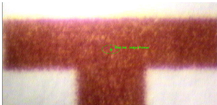
Figure 1: Optical image of one of the samples in the K-Alpha XPS System. The analysis area is defined by the size of the X-ray spot, shown as an ellipse on the image.
