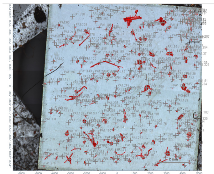
Figure 2. A silicon filter with atmospheric deposition of microplastics. Particles selected are between the size range of 25 \mu\text{m} – 1 \mu\text{m} .
