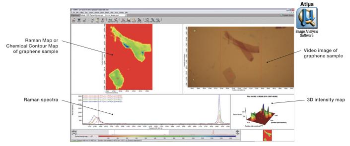
Figure 6. Raman spectra of graphene at specific locations exhibiting differences in layer thickness.
