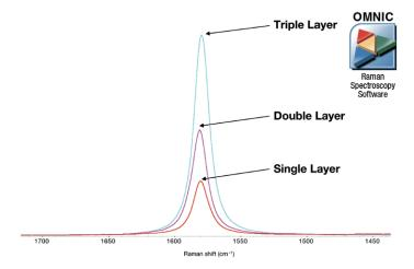
Figure 3. There is a linear increase in G-band intensity as the number of graphene layers increases, collected with 532 nm excitation.
