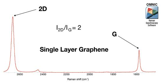
Figure 5. Single layer graphene can be identified by the intensity ratio of the 2D-band to G-band.
