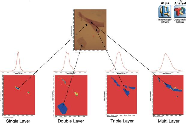
Figure 7. Discriminant analysis applied to the graphene Raman Atlµs Software image shown in Figure 6. The analysis gives the distribution of the different layer thicknesses contained in the sample.
