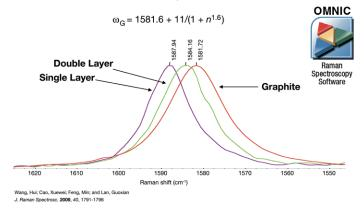
Figure 2. The G-band position is a function of layer thickness. As the number of layers increase, the band shifts to lower wavenumber, collected with 532 nm excitation.
