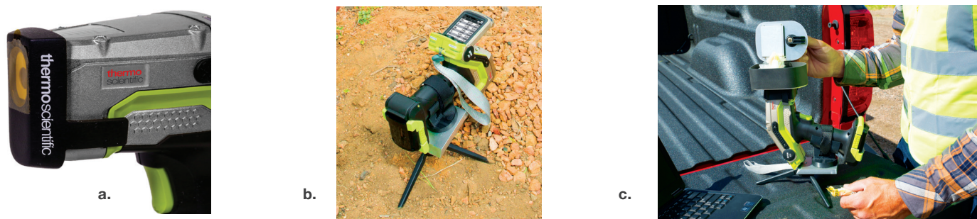
Figure 2. Accessories for the Niton XL5 Plus handheld XRF analyzer: a) Soil guard to protect window bracket b) Tripod for in-situ measurements c) Mini test stand.
