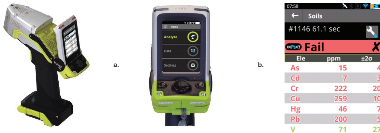
Figure 1. a) Niton XL5 Plus handheld XRF analyzer b) Display of pass/fail result and elemental analysis of soil sample.
