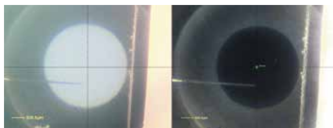
Figure 2: CCD images of the etch crater at the end of the profile, taken using the K-Alpha Reflex Optics and the co-axial lighting with the side lighting (left image) and just the side lighting (right)
