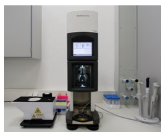
Thermo Scientific™ Vitrobot™ Mark IV System specimen preparation unit for cryo-EM
