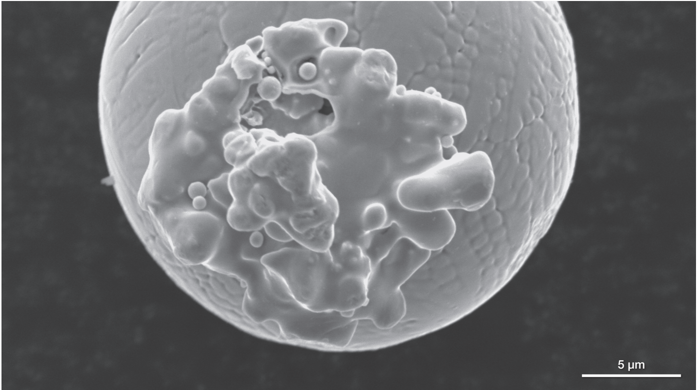
SED image of additive manufacturing powder.
