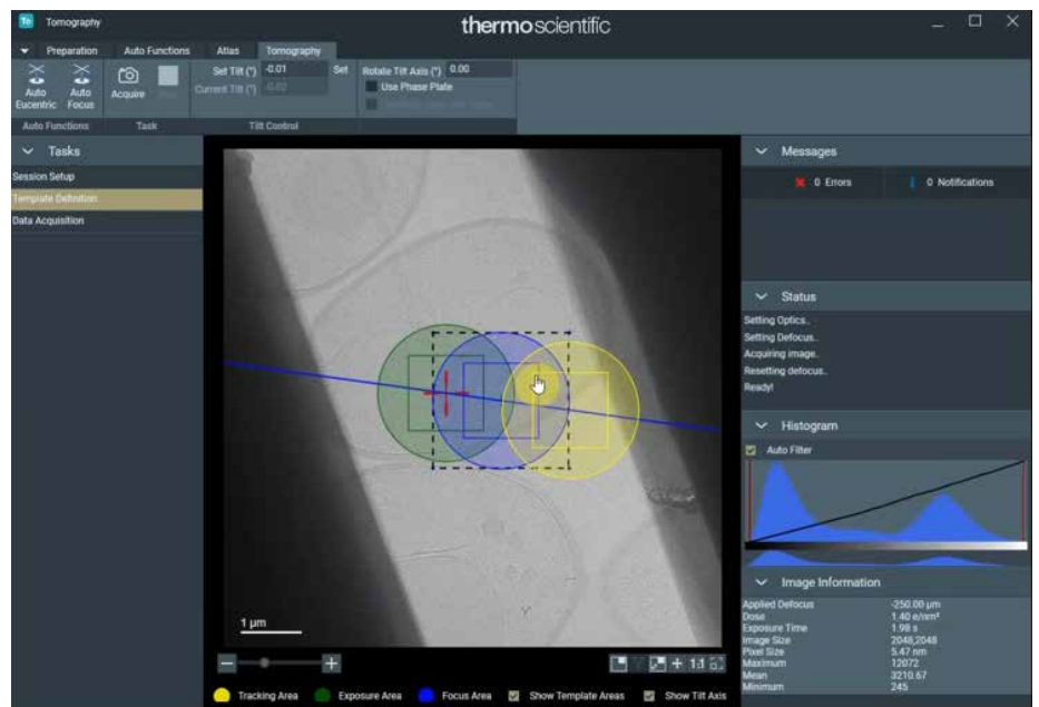
Figure 5. User interface of Tomography 5 Software. Step-by-step settings are made via tabs. User-friendly sections enable users to adjust parameters for each step, view status messages, and display image information. A central viewport allows for display of image data as well as interactive navigation and recording of tomogram areas. Tomography 5 Software is used to assign the acquisition region (green) as well as focus (blue) and tracking areas (yellow) along the tilt axis.
