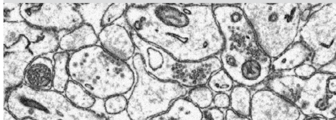
Mouse brain sample. Data acquired by physical slicing at HiVac mode. Imaged in BSE mode at 2 kV accelerating voltage, 0.1 nA beam current, 2 \mu s dwell time. Acquired pixel size 4 x 4 nm. Fine features as vesicles and synaptic clefts can be observed. With permission from Dr. Gabor Nyiri, Institute of Experimental Medicine, Budapest, Hungary.
