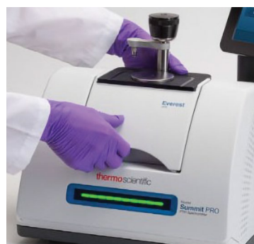
Figure 1. Installing the Everest Diamond ATR in the Nicolet Summit with integrated touchscreen.
