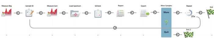
Figure 6: A schematic overview of the final workflow. The workflow, spectra, results, and reports are all automatically saved.
