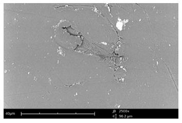
Defect in glass at 2,500x magnification
