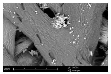
Image of same paper using the charge reduction sample holder. No charging is visible at 5,000x magnification and image details are still clear.
