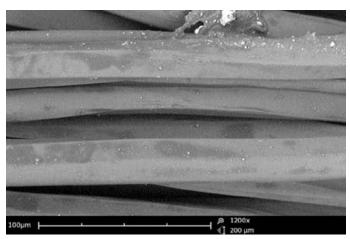
Coated textile fibers at 1,200x magnification
