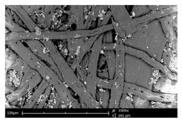
Image of non-conductive paper. The image is taken using the standard sample holder at 1,000x magnification. The bright white areas on both sides of the image is charging. At increased zoom, the charging becomes more localized and more distortion typically occurs until the image is completely obscured, yielding no data.
