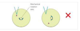
Rotating around an axis that does not coincide with the area of interest causes a shift in position. The user now has to refind the correct (x,y) position.
