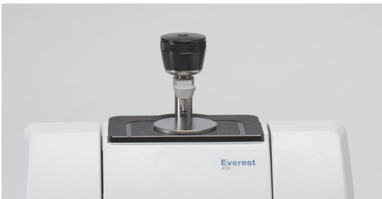
Rotate the pressure tower arm toward the center of the accessory until the tip stops above the crystal. This is the sampling position.
