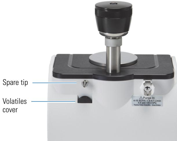
The spare tip and volatiles cover are stored in the back of the accessory.
