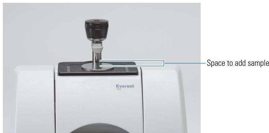
3. Place the sample onto the crystal, directly under the pressure tip.
