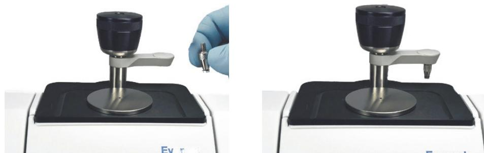
**NOTICE** Do not use tools to install or remove the pressure tip. Using tools may damage the tip.
