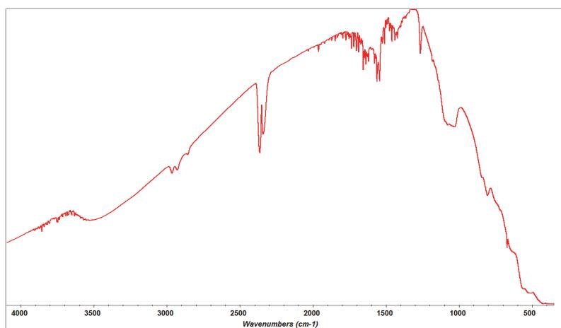
**Note** For troubleshooting purposes and checking for contamination, it is a good idea to save a background spectrum when the crystal plate is new before it has been used for sample analysis.
