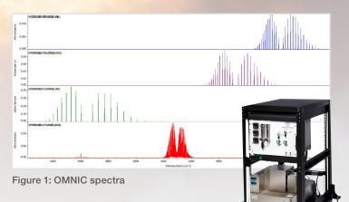
The Thermo Scientific<sup>™</sup> Antaris<sup>™</sup> IGS system, configured with a rackmounted Heated Valve Drawer (HVD), provides a turnkey data acquisition and analysis package (Figure 2). Key features include:
