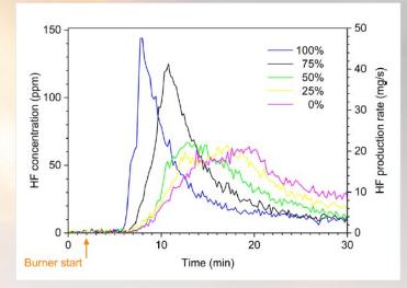
Figure 3: HF gas release from Lithium Ion Battery combustion under different charge conditions. Reference: Larsson, F., Andersson, P., Blomqvist, P. *et al.* Toxic fluoride gas emissions from lithium-ion battery fires. *Sci Rep* **7**, 10018 (2017). https://doi.org/10.1038/s41598-017-09784-z
