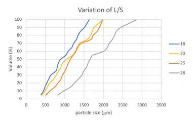
Understanding the influence of the liquid-to-solid ratio has on granule size.
