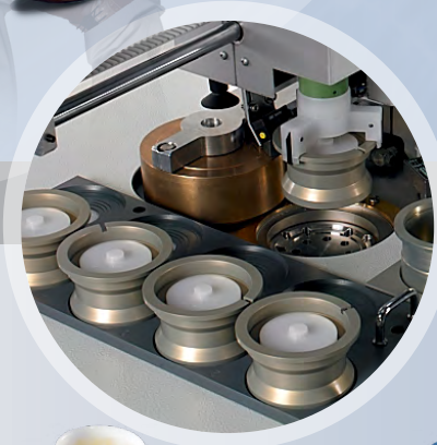
Special cassettes for liquid cell loading
