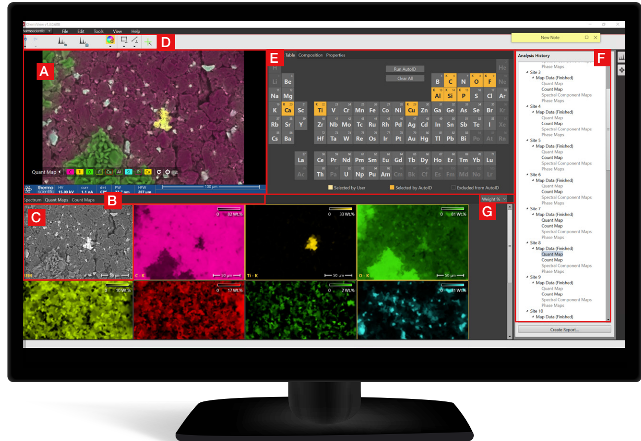
ChemiSEM user interface showing combined SEM-EDS operation in a single display.
