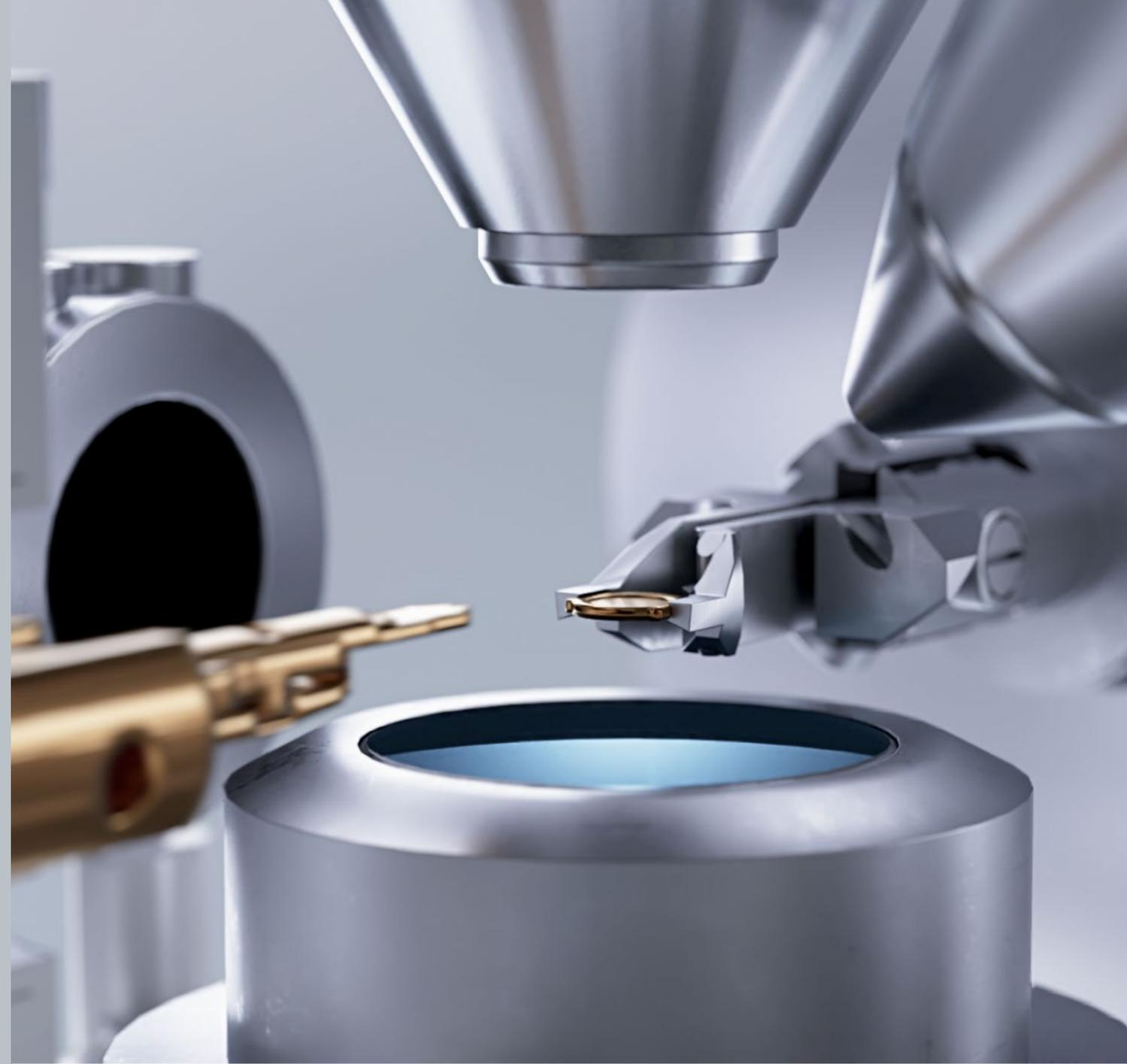
Cryo CompuStage (top right) tilts 180° to image the top and bottom of thick samples. The robotic arm of the Autoloader (top left) provides easy and robust transfer of 12 grids at a time from an Autoloader cassette (bottom left) avoiding unnecessary manual handling and ensuring consistency.
