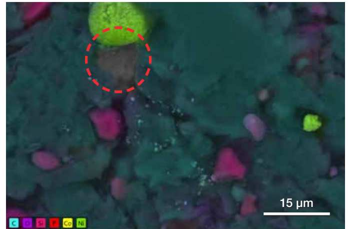
Figure 3: Non-colored area highlighted in red is due to shadowing from a tall feature. Sample: Nickel contamination on a Li-ion battery anode. (20 kV, 4.5 nA, 90 s).
