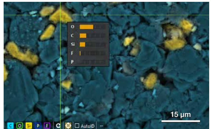
Figure 4: Live tooltip feature. Sample: silicon oxide and graphite Li-ion battery anode. (15 kV, 1.1 nA).
