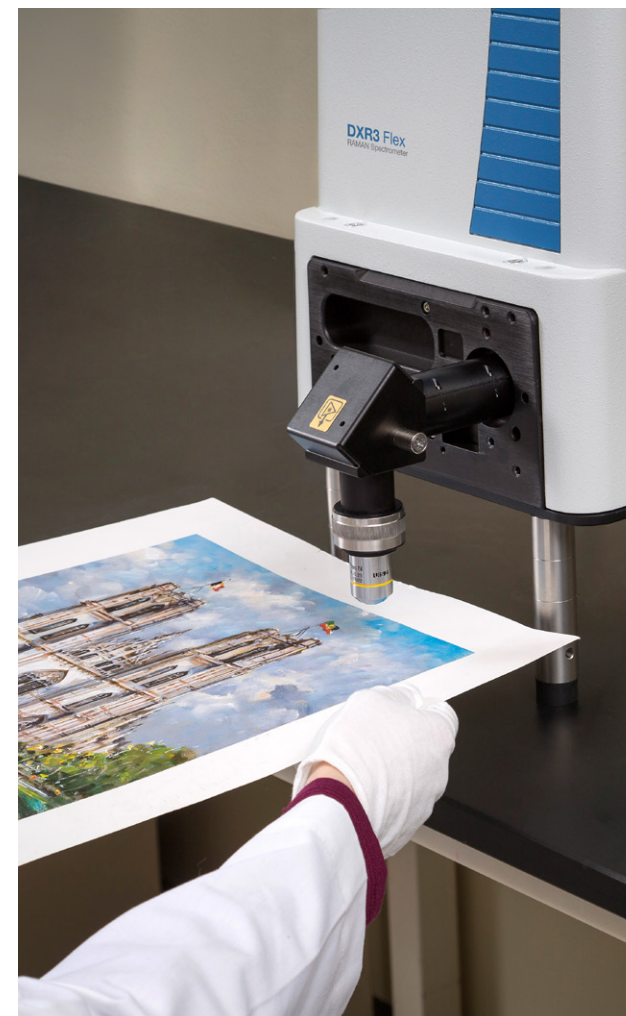
DXR3 Flex Raman Spectrometer equipped with a microscope accessory for art authentication analysis. This eliminates the sample size limit, and with the available lens tube to extend the reach, makes it more accessible for samples of different shapes and sizes.
