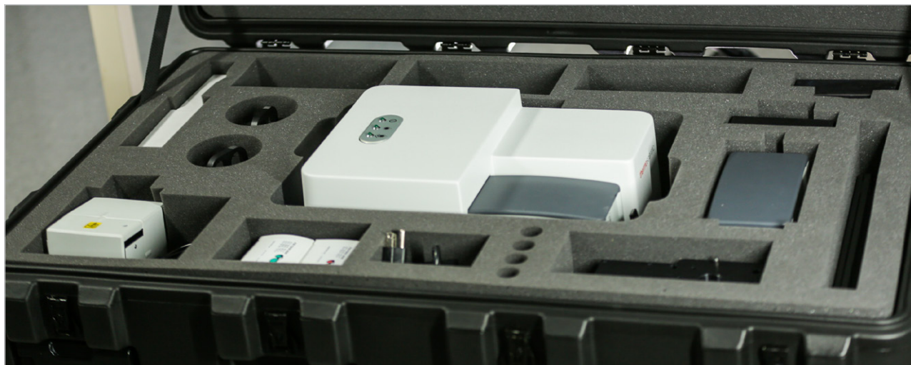
DXR3 Flex Raman Spectrometer and accessories packed in a travel case.
