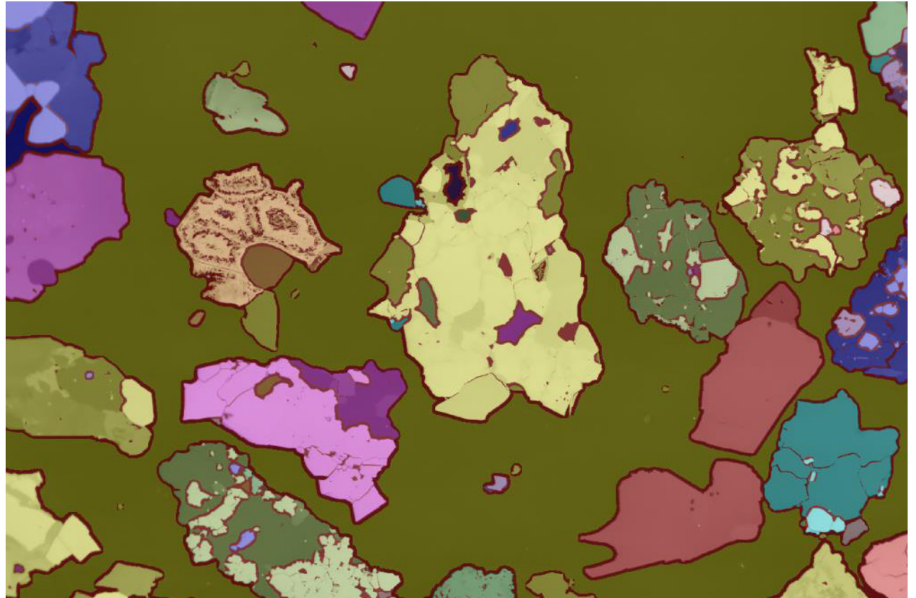
Feature-based image segmentation of a geological sample.
