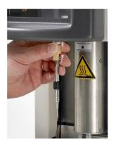
The tweezers with grid are subsequently lifted into the climate chamber by selecting the 'Start Process' button in the User Interface, or alternatively, use the foot pedal switch. The environmental and process parameters (i.e. temperature, humidity, number of blots etc) can now be set as described in:
