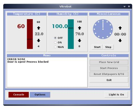
In the console screen the temperature can be set towards any value between 4 °C and 60 °C with the + and – buttons or drag the black marker up or down. The actual temperature read-out is displayed in red.
