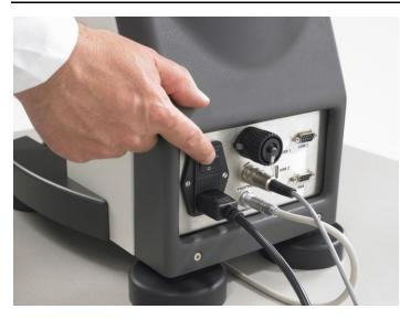
After activation of the hard lock switch the embedded PC with Linux operating system is automatically starting up. The Vitrobot User Interface page will appear after a few seconds.
