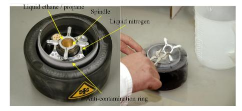
When the ethane/propane container is ready for vitrification the holder can be placed on the platform-ring under the Vitrobot.
