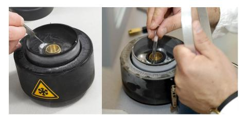
After the grids have been transferred into the grid box, they are sealed with a special screw and usually stored into a somewhat larger dewar for liquid nitrogen prior to the transfer into a cryo holder and subsequently a TEM or SEM.
