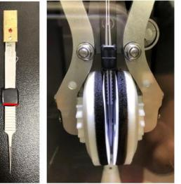
Mount the tweezer onto the connection grove in the central axis. To do this, first select the 'Place New Grid' button in the Vitrobot User Interface to put the central axis in the right position for mounting the tweezer to it.
