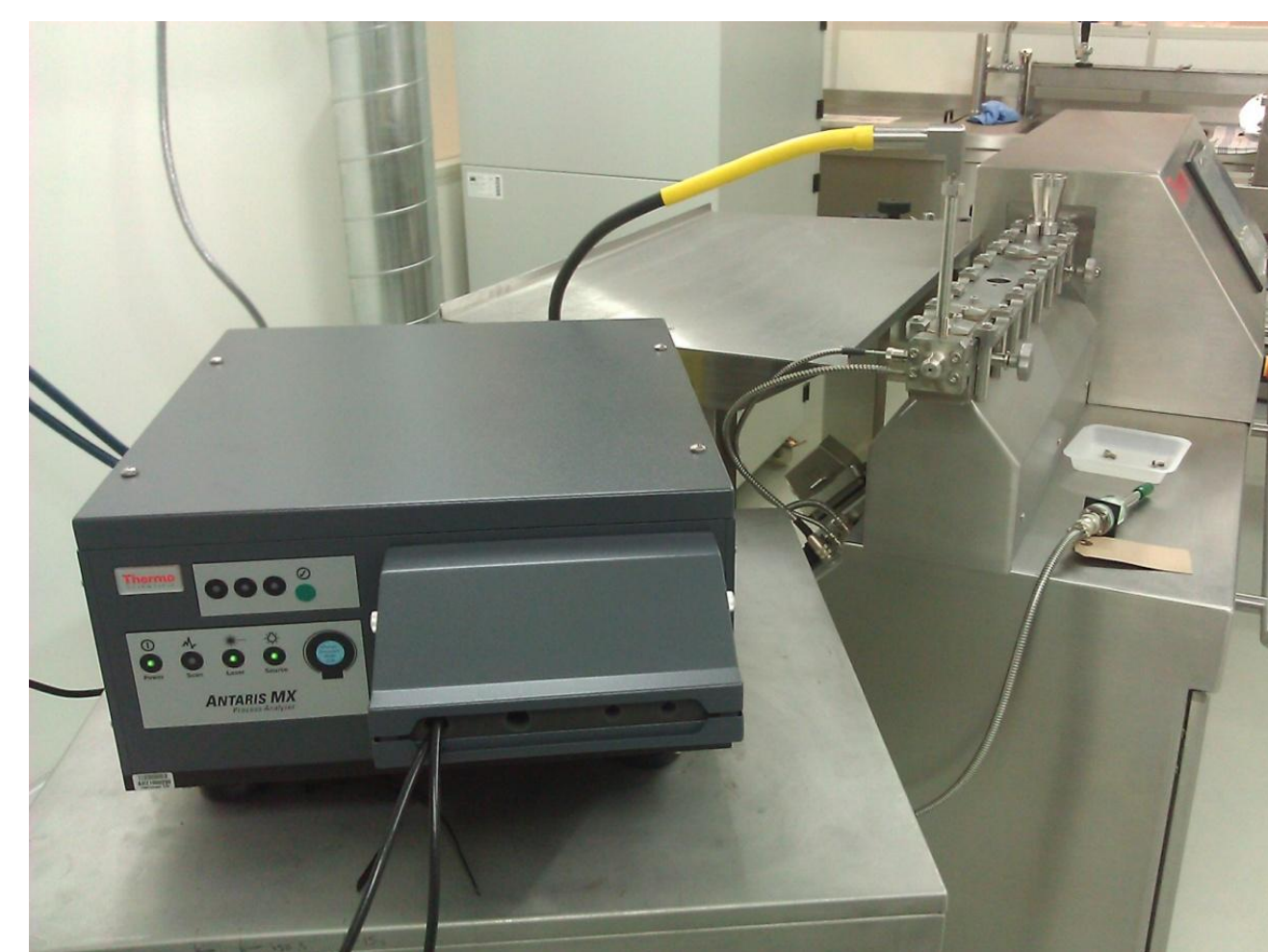
FIGURE 1. Pharma 16 HME Twin-screw extruder with coupled Antaris MX FT-NIR spectrometer
